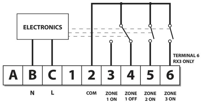
**Note:** 1) For mains voltage operated systems, link terminal 2 to mains live supply
