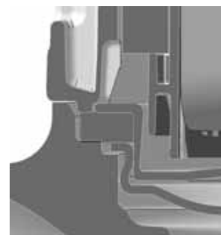
Fig. 37 Sectional drawing showing sealing principle of gasket
